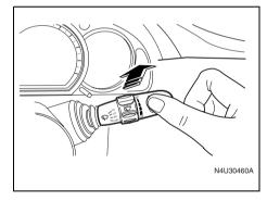
If your vehicle has this feature, operate the rear window washer/wiper system by pushing the windshield wiper/washer lever away from you. The wiper operates continuously when the lever is in the first position. Washer fluid sprays onto the rear window and the wiper operates continuously when the lever is pushed to the second position.
